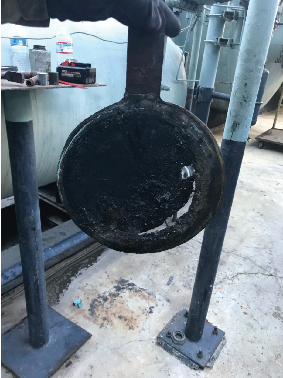
Figure 12. This picture shows the corroded blind slip that was the root cause of fluid entering the out of service pipeline that is buried near surface expression of the leak in the alley.
