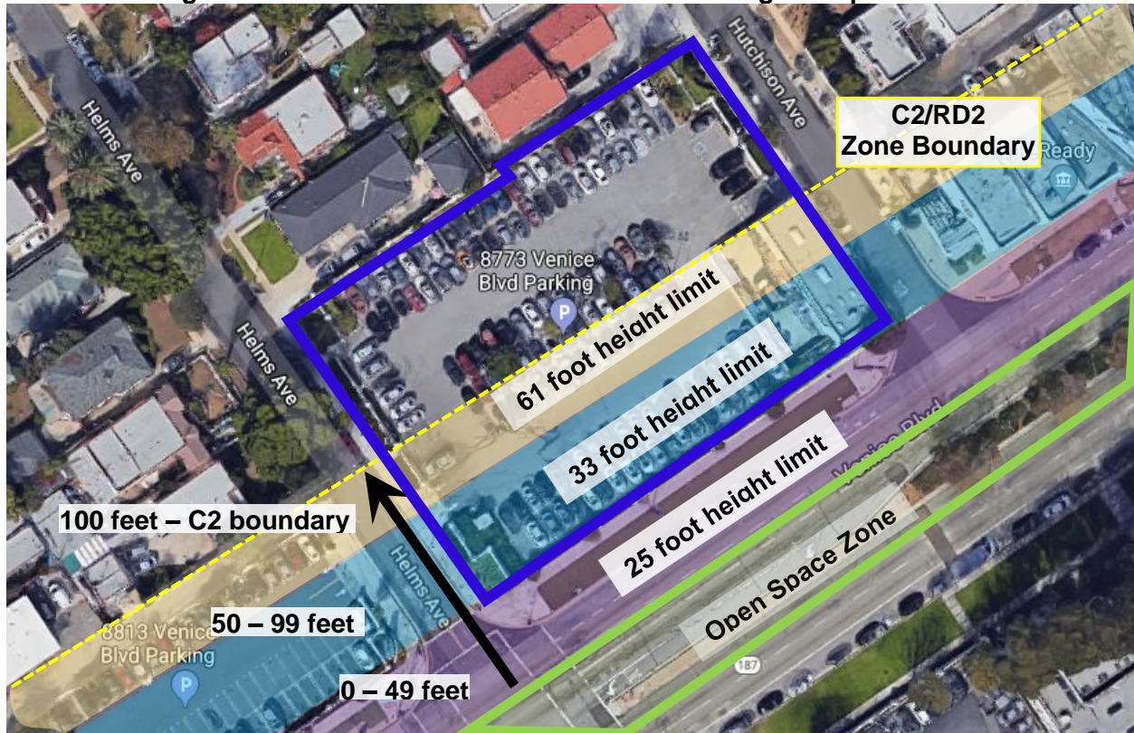
Figure 2. LAMC Section 12.21.1 Transitional Height Requirements
