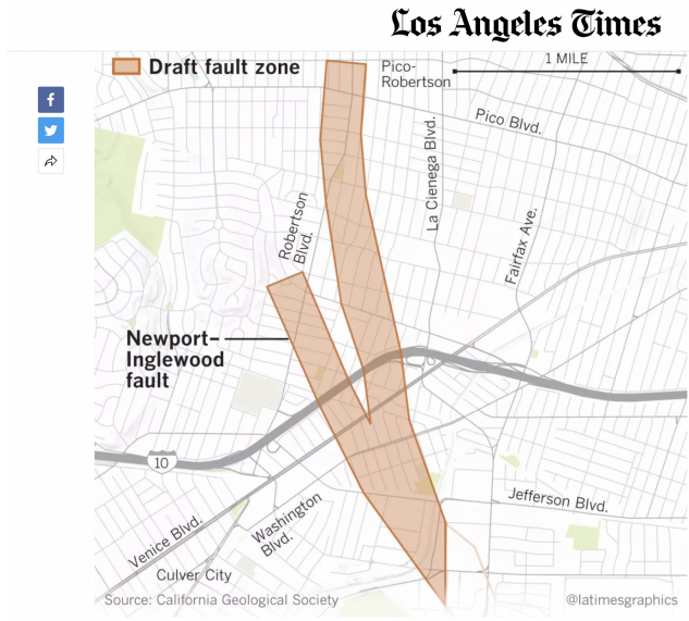
Draft earthquake fault zone map. The area to the south of the shaded area has been previously mapped. (Source: California Geological Survey | Credit: Raoul Rañoa / Los Angeles Times)
